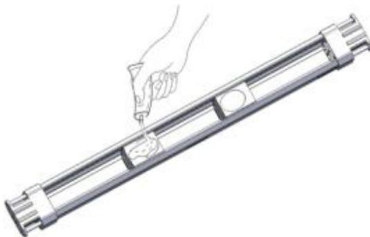
5. According to the fluid flow direction indicated by the bracket probe, fix the bracket probe on the pipe to be measured and twist the sensor downward until it is close to the pipe wall. (See § 4.3.2.3 for fixing method of stent probe).
