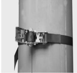
Pull the tensioner spanner continuously to tighten the cloth tape.
