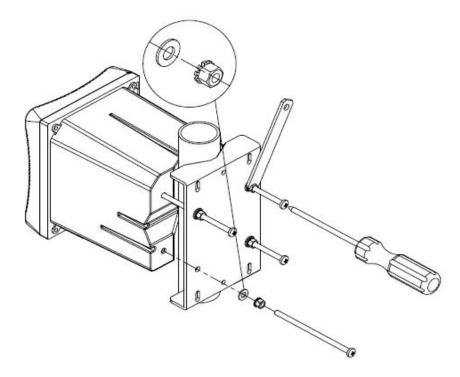
In the installation way of clamp, the diameter of clamp is 1 inch to 2.5 inches.
