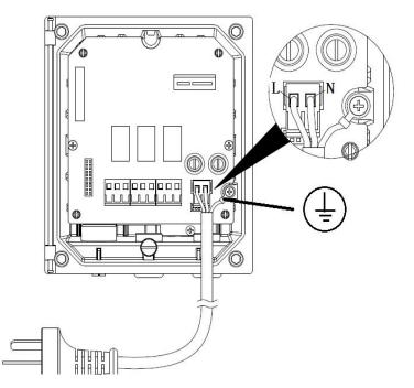
Figure 8 Power Supply Wiring
