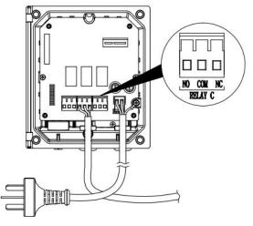
Figure 9 Relay Wiring
